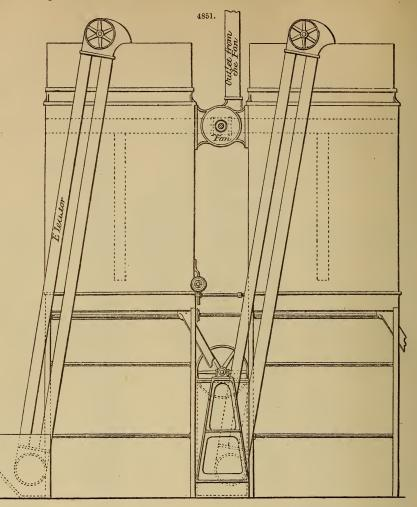
grain from the floor to the top of the first kiln, the other to raise and deliver it to the second kiln. The articles thus pass through both kilns; this is necessary, as peas require to be partially baked. The pair of kilns from which our drawing was taken dry 10 quarters of peas in an hour.
